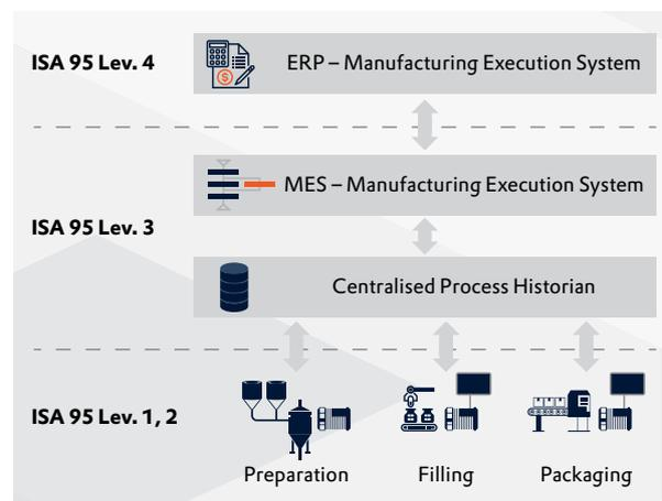
Figure 1: Classic OT - IT integration based on a hierarchical model.
