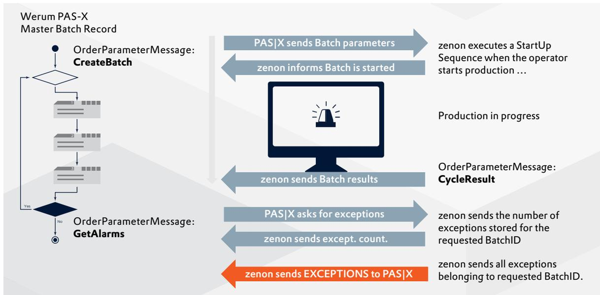
Figure 3: A simple example of communication between PAS-X and zenon for batch management.
