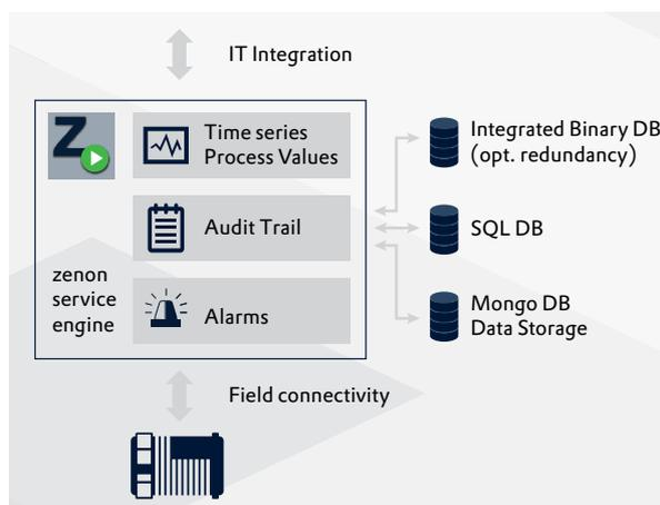
Figure 2: Different storage options using zenon Service Engine.
