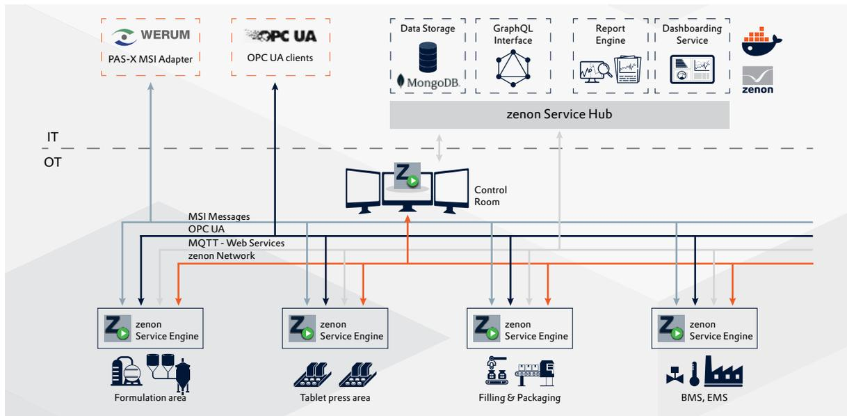
Figure 4: zenon as a modular automation integration layer, including data storage, reporting and IT integration.
