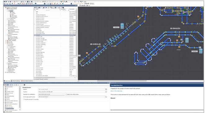
*Budapest Airport’s control system department used the zenon software platform to create a high-level operating system for the air-ground lighting system with its twelve redundant PLCs.*
