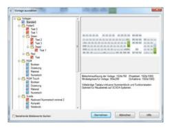
The shipped templates are available in different resolutions and also optimized for touch screens. These templates cannot be changed or deleted. Pre-defined templates by COPA-DATA are saved in the program folder under: \Templates\ScreenTypes\<name of the screen type>\<file name>.zip.
