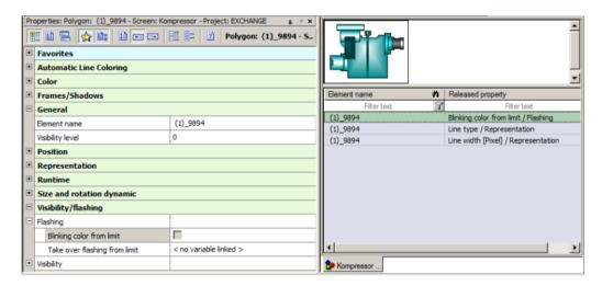
The symbol is edited in the upper area; in the lower area, the released properties of the element of this symbol are listed. You have different possibilities to release elements:
