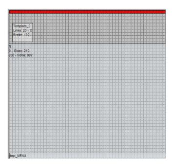
The red frame for the alarm status line is automatically created at the upper edge of the screen by zenon for each project. Its position can be changed via the properties in the Position group. To do this, the Use standard position property must be deactivated.
