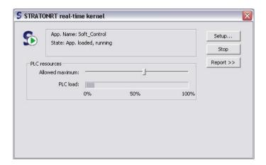
Depending on the size of the PLC application and the defined cycle time the slider has to be adjusted to the PLC load. The slider can be set between 10% and 85%. The current load (bar) indicates whether the allowed maximum for executing the PLC cycle is sufficient.
