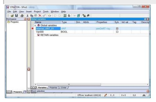
Such a variable is especially marked in zenon Logic, as it cannot be changed in zenon Logic. Changing the variable here would lead to problems, as the source of the variable is the PLC programming environment in the external PLC (e.g. S7).
