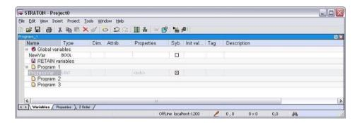
Mark the line Properties of the corresponding variable. Press Ctrl+F12. Thus the profile zenon Logic is displayed in this line. In addition you must activate the checkbox for embedding the symbol via double click or Enter in column symb...
