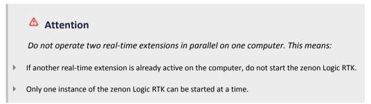
The Realtime Kernel is designed, so that it triggers the zenon Logic Runtime cycle independent of Windows. So the zenon Logic Runtime cycle is guaranteed to be executed deterministically. Cycle times must be  $100 \, \mu s$  or higher.
