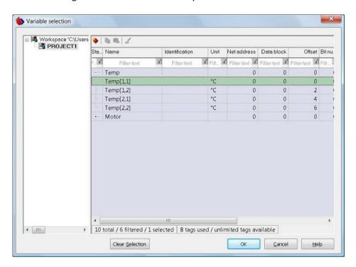
▶ In the dialog box Variable selection, highlight the variable Temp[1.1] and then press the button ox.
