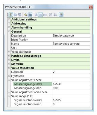
► Change the properties Unit, Decimals, Linear value adjustment and Value range PLC of the datatype as shown in the illustration above.
