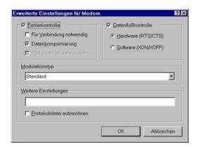
there is a checkbox for recording a log file. If it is activated, all data exchanged with the modem are recorded in a log file. The file is in the Windows directory (e.g. C:\WINNT) and has the name of the modem, for which logging is activated. e.g.: ModemLog\_Sportster 28800-33600 External.txt. This file is useful to find errors. Because of the quickly growing size logging should only be activated for a short time.
