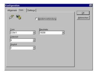
configuration dialog Com. If the checkbox Modem connection is available, the driver can connect to the PLC via modem.
