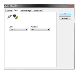
For this driver, only COM port and baud rate for the communication can be changed. All other communication parameters are defined and fixed in accordance with the IEC 870-5-101 standard.
