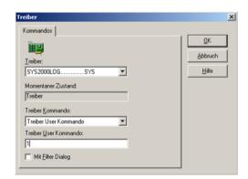
The default value P=1 means that the automatic checking is turned on; the driver polled the stations whether connections are active and whether values are available. With value P=0 you turn off the automatic checking.
