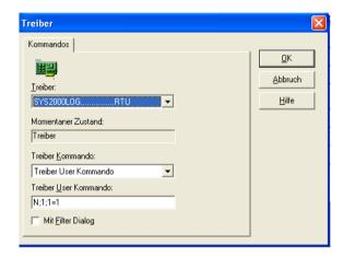
With T;NetNumber;NodeNumber (e.g. T;1;1) you can transfer the local time of the computer to the PLC. With P=0/1 the polling is activated (1)/deactivated (0). Automatic recognition of a calling station: By default, there is a cyclical check, whether there has been a call to the PC via modem by a station, for which RDA data was defined. If this is the case, all values are read out automatically and sorted into the archives. This automatic check can be disabled with a driver user command.
