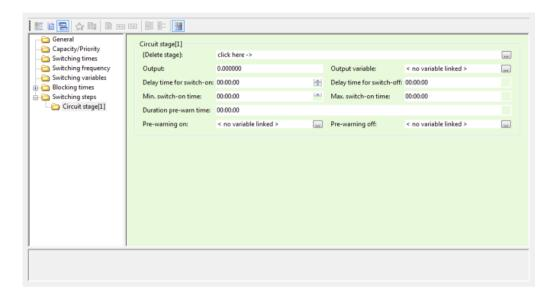
Each switching level offers settings for the output, the forewarning of the switching and the switch-on and switch-off. All adjustable properties are described in the help window after you click on them.
