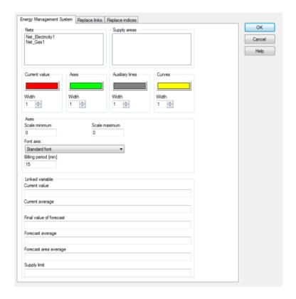
In the Runtime the EMS screen is opened with the help of a screen switch function. For the screen callup the following parameter can be set:
