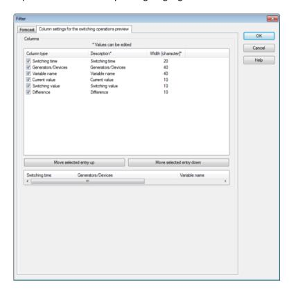
In the list field of this tab all available column types are displayed. With the help of a checkbox you decide which column types are displayed. You can change the description and the width of each column type by left-clicking the corresponding area and entering the desired value in the input field.
