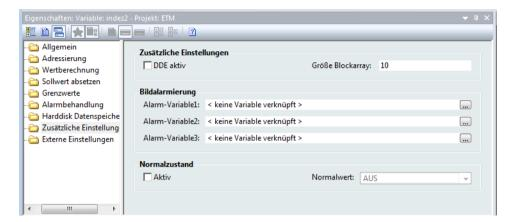
▶ Select, for the screen switching function, the array data property on the ETM screen:
