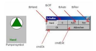
In this example we draw a pump consisting of a circle and a triangle. Define the triangle as a symbol. On top draw a multibinary element and link it to three bit marker variables.
