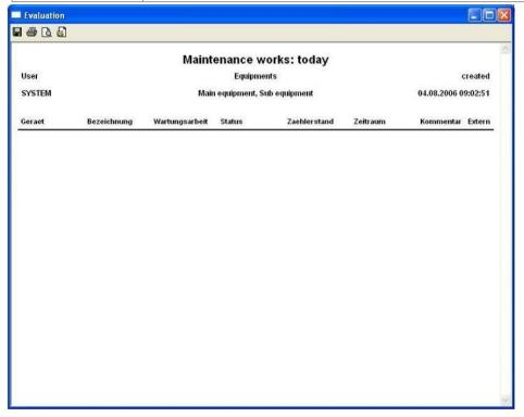
The displayed list is written to am XML file as it is and displayed in a HTML browser with a stylesheet. This HTML file then can be saved or directly printed.
