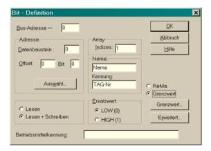
When defining this variable, enter the target module as "net address".
