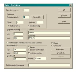
When defining this variable, enter the target module as "net address".
