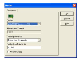
With T;NetNumber;NodeNumber (e.g. T;1;1) you can transfer the local time of the computer to the PLC. With P=0/1 the polling is activated (1) or deactivated (0). Automatic recognition of a calling station: By default, there is a cyclical check, whether there has been a call to the PC via modem by a station, for which RDA data was defined. If this is the case, all values are read out automatically and sorted into the archives. This automatic check can be disabled with a driver user command.
