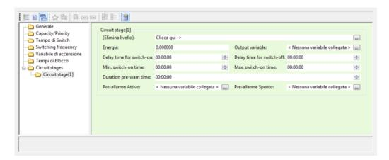
Each switching level offers settings for the output, the forewarning of the switching and the switch-on and switch-off. All adjustable properties are described in the help window after you click on them.
