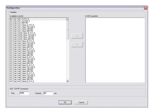
Here the variables that should be connected can be selected. In the list on the left-hand side all variables which are available in zenon are displayed. These can be selected and moved to the DEC export list with the '>' button. With the button '<' they can be removed again. If a variable is moved to the export list, a dialog for the name assignment of the zenon variable to the DEC variable opens:
