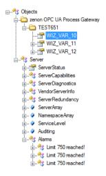
The screen shot displays the inclusion of the zenon project (TEST651) and the zenon variables (WIZ\_VAR\_10, WIZ\_VAR\_11, WIZ\_VAR\_12) as objects in the upper area. This includes the alarms when the limits set up have been reached (Limit 750 reached! etc).
