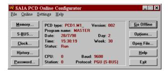
The settings for the modem-communication are done in this "PCD Configurator". Notice: Settings can only be changed, if an online connection to PCD exists.
