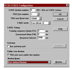
In this dialog, the settings are done analogically. Configuration of the modem type depends on the manufacturer. Click on the Button "Modem" to insert the Modem string. To access further S-Bus-Stations, activate the "Gateway". The exact configuration is described in the SAIA handbooks. The settings are stored in the "Spg4modm.ini" file. This file must be stored in the Windows directory.
