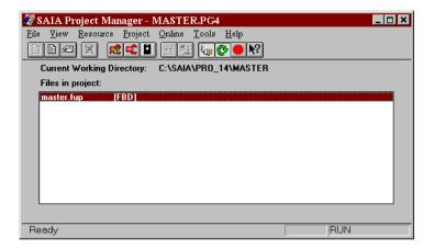
In the "Project manger" under "Tools" the "PCD Configurator" is started.
