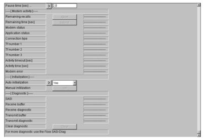
The settings of the Modem depends on the Modem manufacturer. The settings are saved in "modmsms.def" in the folder \*\\SAIA\\FBox\\\*. How the settings have to be done is explained in the SAIA handbooks.
