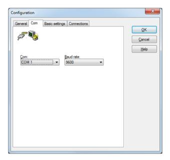
For this driver, only COM port and baud rate for the communication can be changed. All other communication parameters are defined and fixed in accordance with the IEC 870-5-101 standard.
