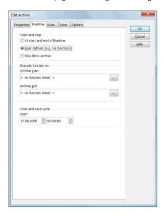
▶ Set Start and end to User defined, so that we can start and stop the lot archive by hand (i.e. with functions) with the start and end of the production cycle.
