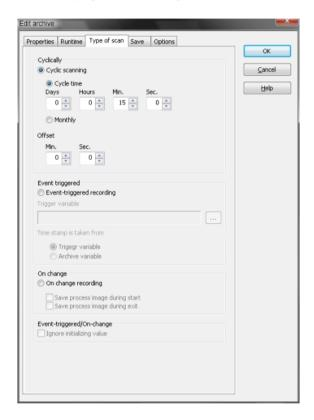
No settings are needed here. Aggregated archives are also recorded on change. zenon recognizes the archive as an aggregated archive and automatically sets the scan type to on change. The scan rate is defined with the length of the basic archive files.
