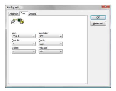
According to IEC62056, the following interface parameters are to be used:
