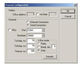
PGU must not be activated here; otherwise, the PCD2 will switch immediately to P800 mode. If PGU is deactivated, S-BUS will be used for communicating.
