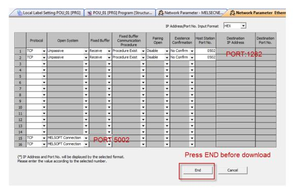
For Ethernet connections: tested with SPS MELSEC Q series and QJ71E71-100
