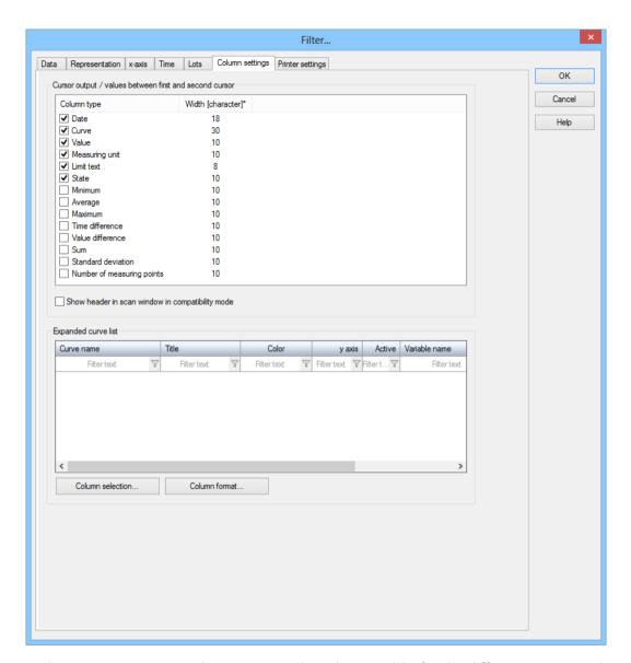
In the Column settings tab, you can set the column widths for the different entries in the cursor output window. With the help of the checkbox you decide which columns you want to display.
