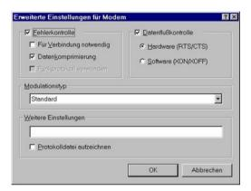
there is a checkbox for recording a log file. If it is activated, all data exchanged with the modem are recorded in a log file. The file is in the Windows directory (e.g. C:\WINNT) and has the name of the modem, for which logging is activated. For example: ModemLog\_Sportster 28800-33600 External.txt. This file is useful to find errors. Because of the quickly growing size logging should only be activated for a short time.
