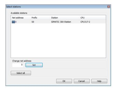
Select the desired stations (CPU) in the following dialog. The dialog supports multi-select. You can select several functional charts at once if you press and hold Ctrl or Shift while making your selection. You can set the net address for communication here. Confirm the dialog with **OK**. An analysis of the S7 project is carried out. Depending on the size of the project, it can take some time.
