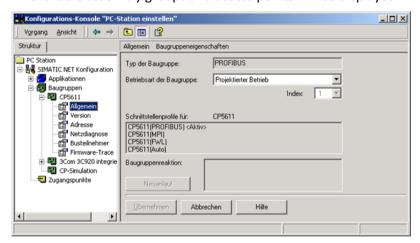
**Important:** The operation type of the assembly group must be set to "Configured operation".
