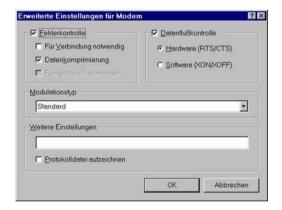
there is a checkbox for recording a log file. If it is activated, all data exchanged with the modem are recorded in a log file. The file is in the Windows directory (e.g. C:\WINNT) and has the name of the modem, for which logging is activated. For example: ModemLog\_Sportster 28800-33600 External.txt. This file is useful to find errors. Because of the quickly growing size logging should only be activated for a short time.
