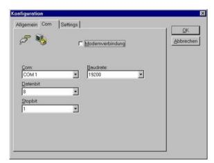
configuration dialog Com. If the checkbox Modem connection is available, the driver can connect to the PLC via modem.
