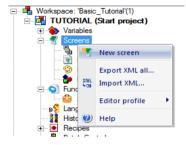
A screen with the name "Screen 0" is automatically created. You can change the properties of the screen in the property window.
