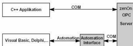
The COM interface is used by function-pointer-orientated languages, such as C++. It is possible to communicate with script languages, such as Visual Basic, using the Automation Interface.
