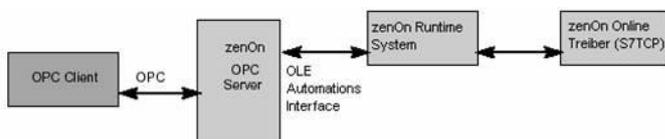
OPC defines objects that are described by object interfaces. In the OPC server there are two kinds of object interfaces, which can be addressed by an OPC client:
