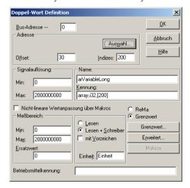
You can also place an array variable in the control system over a B&R PLC structure. This means that an unformatted binary dump of the structure will be read and written.
