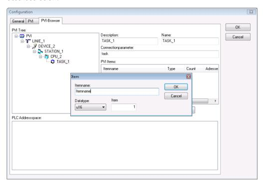
With the button "Browse" the list window PLC Addressspace is filled with the data from the PLC. In order to create single PVI items they can be imported by double-clicking them.
