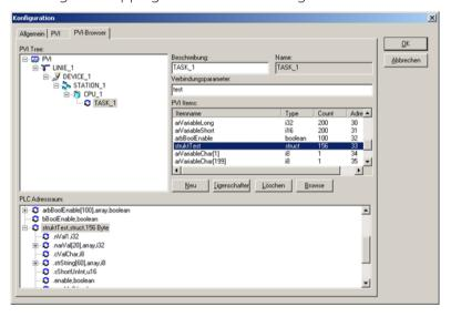
2. Creating the variable in the control system: by clicking the Select button, you can select the mapping variable created above from a list (only works for type i8/u8).
