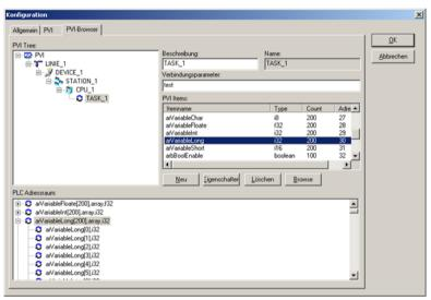
2. Creating the control system variable: by clicking the Select button, you can select the mapping variable created above from a list.
