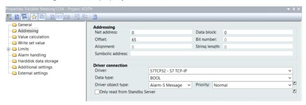
For **Alarm\_8** messages, the index of the message must also be entered in the **Data block** property. This corresponds to the index of the **Alarm\_8** module input to which the message is generated (0 -7).
