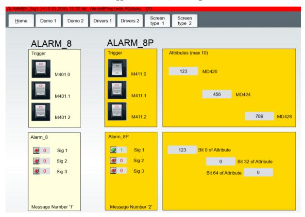
The associated value of the **Alarm-8P** block is sent with the message and displayed using the associated variables (attributes).
