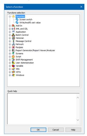
A function is created after you have selected it and confirmed with **OK**. The parameters of this new function can now be defined in the properties window.
