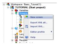
A screen with the name **Screen 0** is automatically created. You can change the properties of the screen in the properties window.
