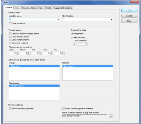
If **this dialog is offered in Runtime** deactivated, screen switching is carried out immediately in Runtime with the filter settings set (in the Editor) for the respective screen.
