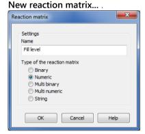
In the **reaction matrix** dialog that opens, enter *Fill level* as the *name* and **Numerical** as the *type*.
