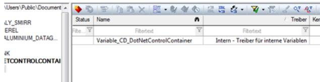
2. In the zenon project node *Project/Files/Others* add the DLL of the created .NET user controls. Here, the file is copied to the **Additional** file at file system level.
