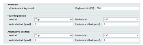
This setting is not activated by default. When activating, the automatic keyboard is created by the system and is automatically called up in Runtime relatively close to the element. It appears where a set value is to be entered. You can configure your own properties such as size or position by means of the properties in the Editor.
