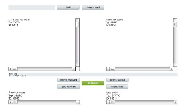
The screen of the *Process Recorder* type is for controlling playback of recorded process data in Runtime.
