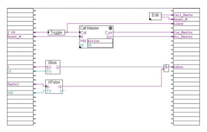
The illustration shows another example program, in which a communication from SAIA PCD to zenon can be established. In the "Call Master" Component the selection settings are done.
