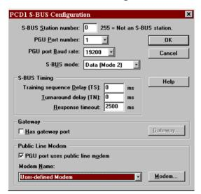
In this dialog, the settings are done analogically. Configuration of the modem type depends on the manufacturer. Click on the Button "Modem" to insert the Modem string. To access further
