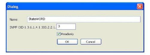
The variables selected in this way are then available on the SNMP server and are continuously synchronized between zenon and the SNMP OID structure. For every OID address you can define whether it can be write-accessed via SNMP SET. The exact structure of every OID address is described in the chapter "MIB structure.
