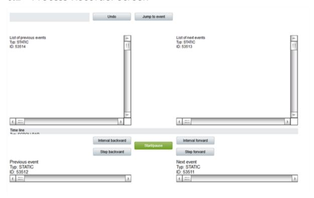
The screen of the *Process Recorder* type is for controlling playback of recorded process data in Runtime.
