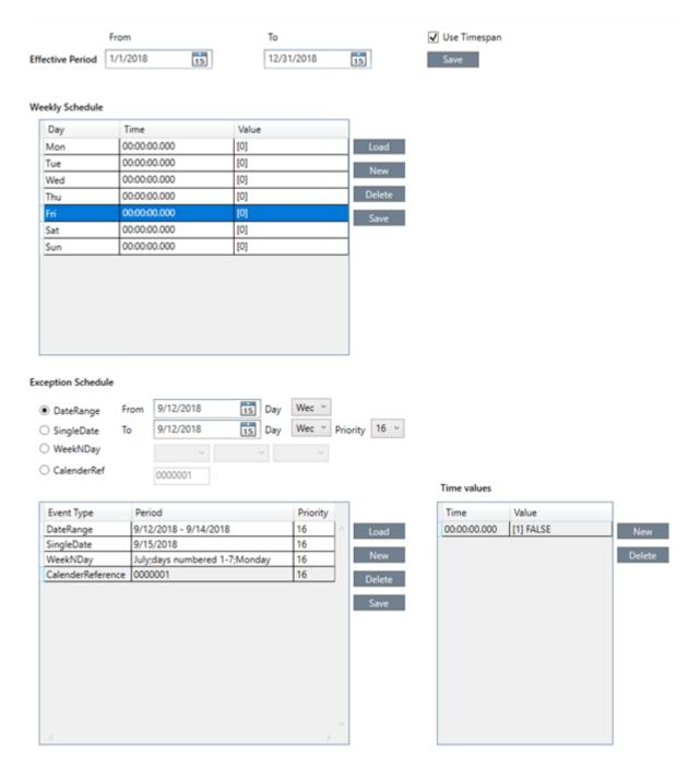
In zenon Runtime, existing BACnet schedule objects can be read by the PLC, modified in the Runtime and saved back to the PLC.
