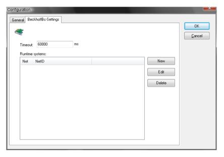
On the "BeckhoffBc settings" page, you can assign the used AMS net addresses to a hardware index. With this hardware index, you can specify the device on which a variable resides.
