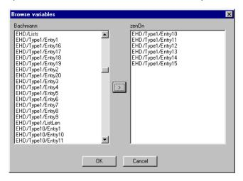
Use the ">" button to move all entries selected in the list of the LogiCAD variables into the list of variables that will be imported into the control system (multiple selections can be made with the Ctrl key and the Shift key). Click OK to import all entries in the control system list into the project. At the moment, only the name and the type will be imported.
