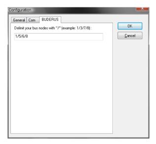
Enter all addresses of the modules connected to the ECOCAN BUS in the box.
