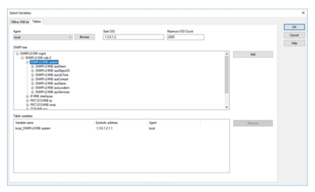
In this dialog, the driver reads data from the SNMP agent. The content is stored in a STRING variable of the **SNMP table** driver object type.
