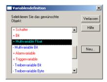
For example to read the "H" parameter of sensor 1, a variable of the type "multivariable float" has to be created.
