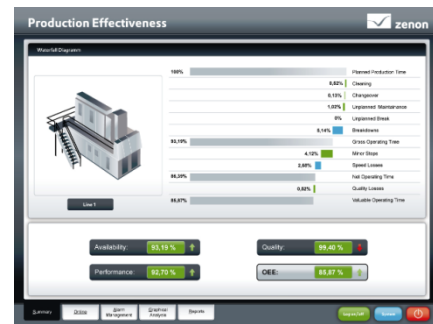
Analysis using an OEE Waterfall Diagram in zenon
