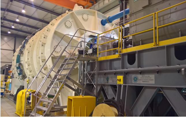
*Instytut Lotnictwa’s new test facility allows for challenging tests on jet engine fans.*
