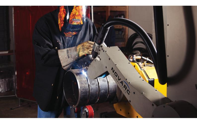
Novarc Technologies designs and manufactures pipe welding machines and welding automation technology. The Canadian start-up, based in North Vancouver, British Columbia, was established in 2013 and has attracted substantial investment thanks to its innovative collaborative spool welding robot (SWR).
