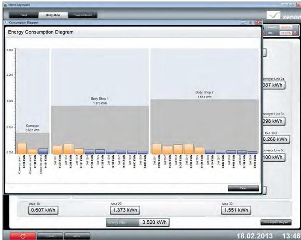
The dynamic bar of current energy consumption recognizes deviations within the systems at a glance.
