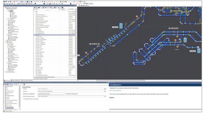
The visualization for the baggage handling system with its more than 1,000 conveyors was created in two weeks purely by parameter setting.
