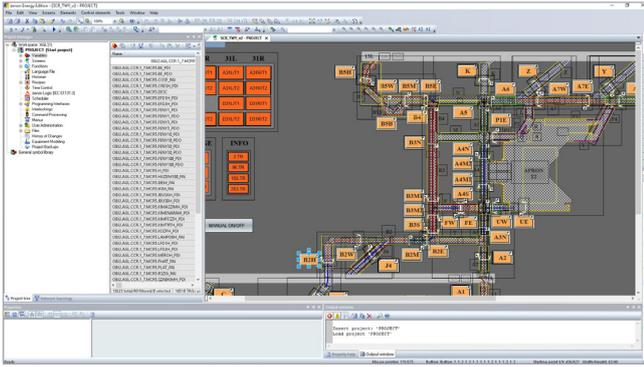
Budapest Airport’s control system department used the zenon software platform to create a high-level operating system for the air-ground lighting system with its twelve redundant PLCs.
